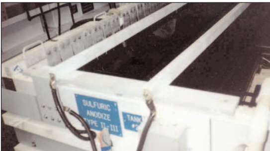
Anodizing is a water-based process and uses no volatile organic compounds (VOCs).
